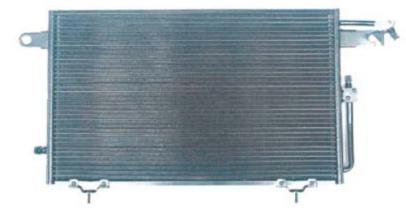
The Condenser function is to act as a heat exchanger and allow heat to flow from the hot refrigerant to the cooler outside air.
